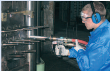
Mould cleaning on hot moulds
