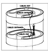
Multilayer system for degrees up to 1440°.
