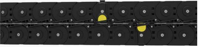
Through **Brevetti's i-Roller mechanism**, rollers at the lower chain portion are protruded and the upper chain portion slides along a perfectly smooth surface.
