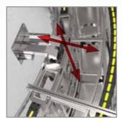
The movable point is equipped with a cable conveyor and a tow arm designed to compensate for vertical and radial misalignment.
