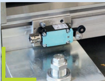
Limit position detection and area monitoring with roller lever switch
