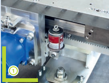
Lubrication of the drive unit with cartridge system for increased service life
