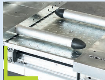
Collision protection mechanically and with sensors
