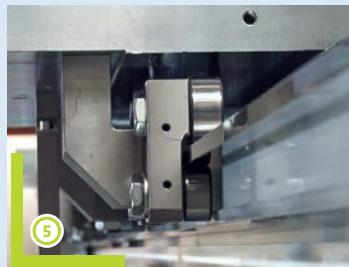
Carriage with roller guide for easier maintenance
