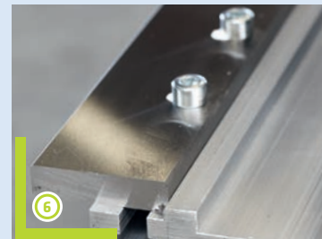
Guide rails hardened and ground for repeatability and positioning accuracy
