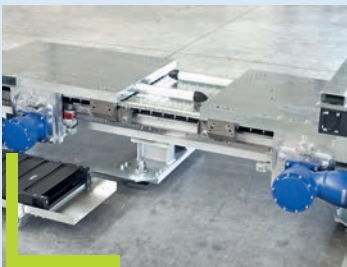
Additional carriage with gear box
