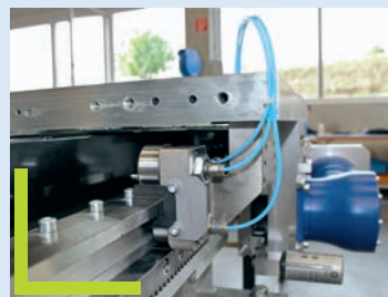
Central lubrication of rollers for easier maintenance
